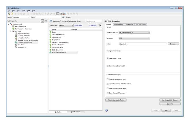
In the code generation exercises that follow, you use the Configuration Parameters dialog box to view and set HDL Coder options and controls. The exercises use the sfir\_fixed model (see "The sfir\_fixed Model" on page 3-14) in basic code generation and verification steps.
