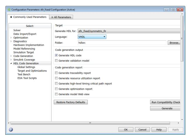
The following figure shows the top-level  $\mbox{HDL}$   $\mbox{Code}$   $\mbox{Generation}$  options pane in the Model Explorer.
